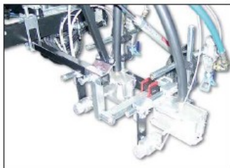
Code 4500: PEARLIZED REFLECTING PAINT DISTRIBUTION
